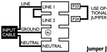
**Note:** For systems manufactured before 1999, if P33 & P34 are missing, install a 4-mm dia. cable between Line 1 and Line 2.
