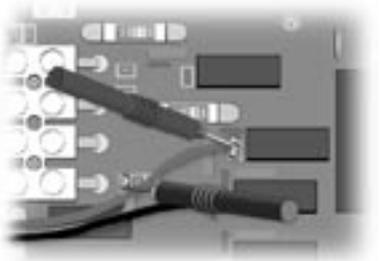
Turn Pump 1 to high speed and take voltage reading between blue and brown wire connectors (P7 & P12).
